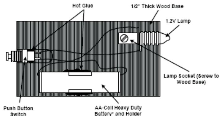
\*Use only a battery labeled "Heavy Duty". Alkaline, etc. batteries will burn out the lamp in a few minutes.
